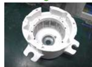
Winding assembly parts after BMC molding
